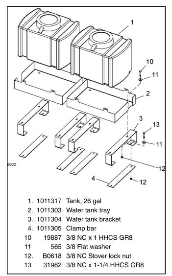
Figure 7. Water Tank Installation
